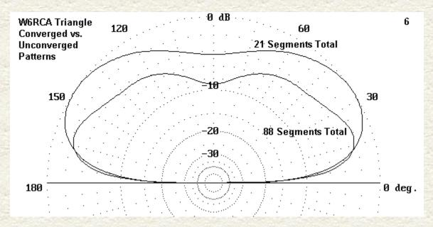
Unlike the right-angle delta, the W6RCA triangle can be modeled via MININEC, since the bottom is about 0.22 wavelengths above ground. Even though MININEC advises against modeling with small numbers of segments when an antenna geometry contains right or acute angles, the exercise may be instructive. Again, for this example, the model is split-current fed.
